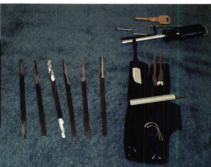
A set of various rocker picks on the right, and A-1's set for picking the GM 10 cut ignition on the left.
