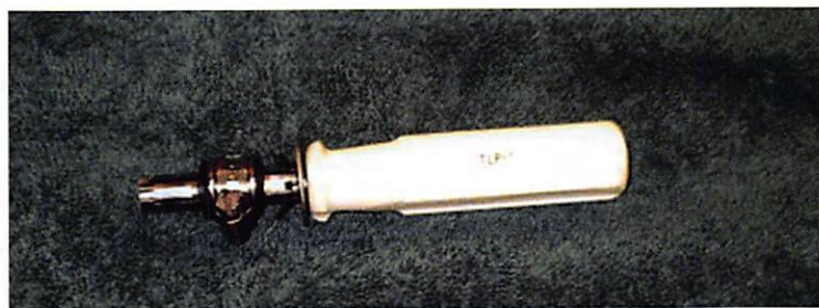
A common tubular pick, but with a piece of hose and a small hose clamp to provide minute adjustments to the tension.
